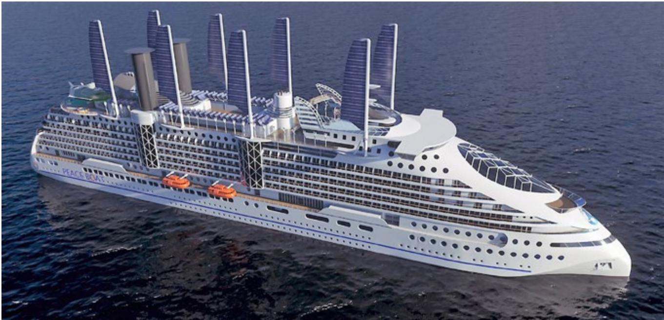
Peace Boat ECOSHIP con los paneles solares en forma de velas desplegados | Peace Boat ECOSHIP with shaped solar panels of sails unfurled
